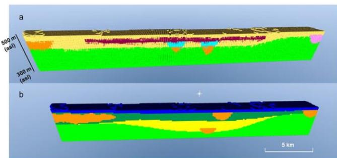
**Figure 3.** (a): Voxel model constructed from updated waveform with a-priori (ERT) information incorporated; (b): voxel model based on original VTEM inversion results.
