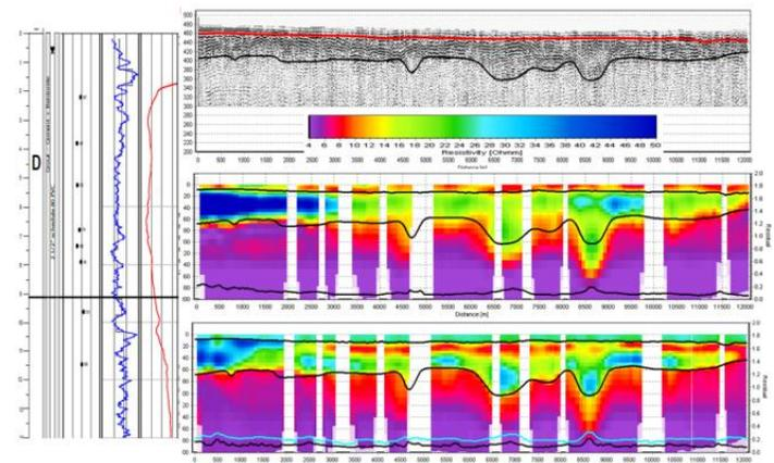
Figure 2. Top: Seismic section with interpretation; middle: original VTEM inversion; bottom: recalibrated VTEM inversion (Aarhus Geophysics); left: downhole resistivity log.
