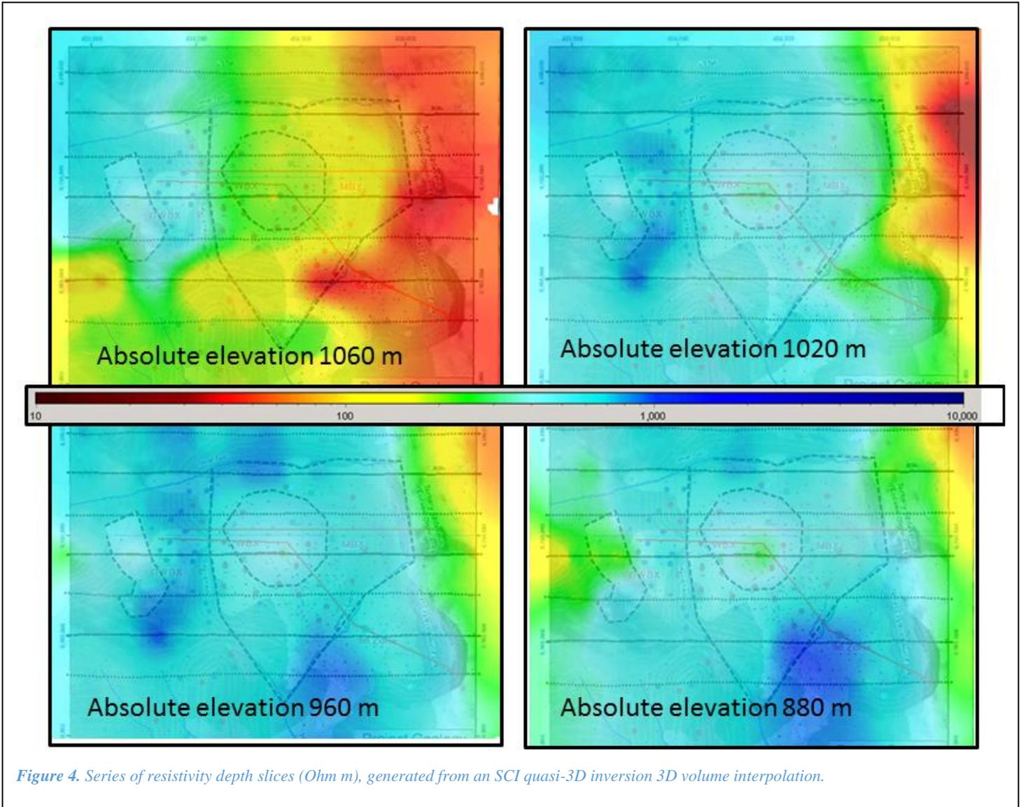
Figure 4. Series of resistivity depth slices (Ohm m), generated from an SCI quasi-3D inversion 3D volume interpolation.
