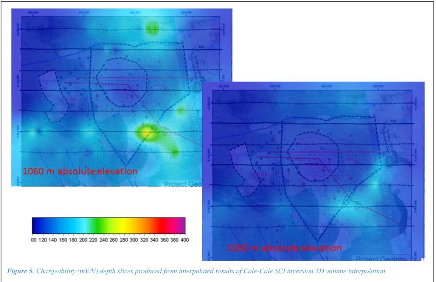
Figure 5. Chargeability (mV/V) depth slices produced from interpolated results of Cole-Cole SCI inversion 3D volume interpolation.
