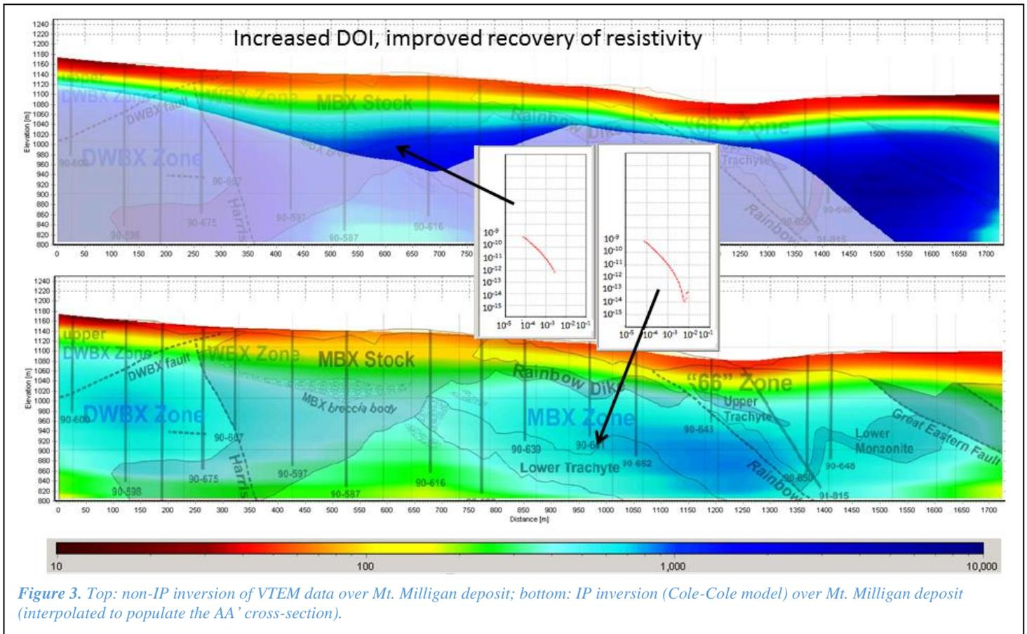
results. Not only the IP inversion brings greater depth of investigation and improved recovery of electrical resistivity, but in the case of the Mt. Milligan deposit, the ability to extract chargeability plays a crucial role, since the deposit is electrically resistive and chargeability becomes a primary quality in overall detectability of the deposit (Oldenburg et al., 1997).
