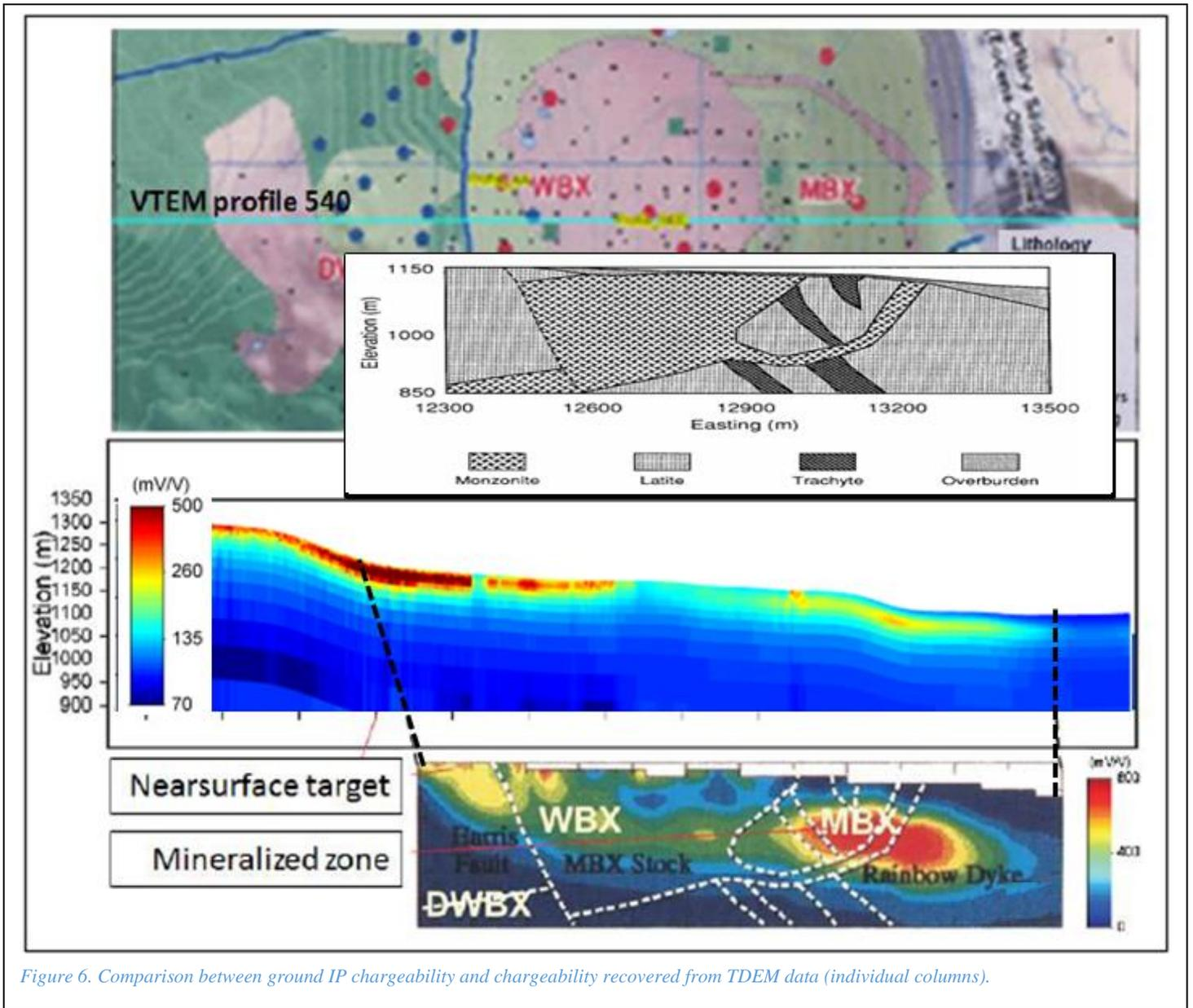
Figure 6. Comparison between ground IP chargeability and chargeability recovered from TDEM data (individual columns).
