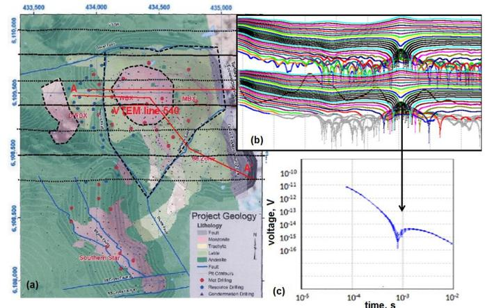
Figure 2. (a): Bedrock geology of Mt. Milligan deposit. (b): visible IP effect in VTEM data (flight line 540). (c): IP effect in individual transients.
