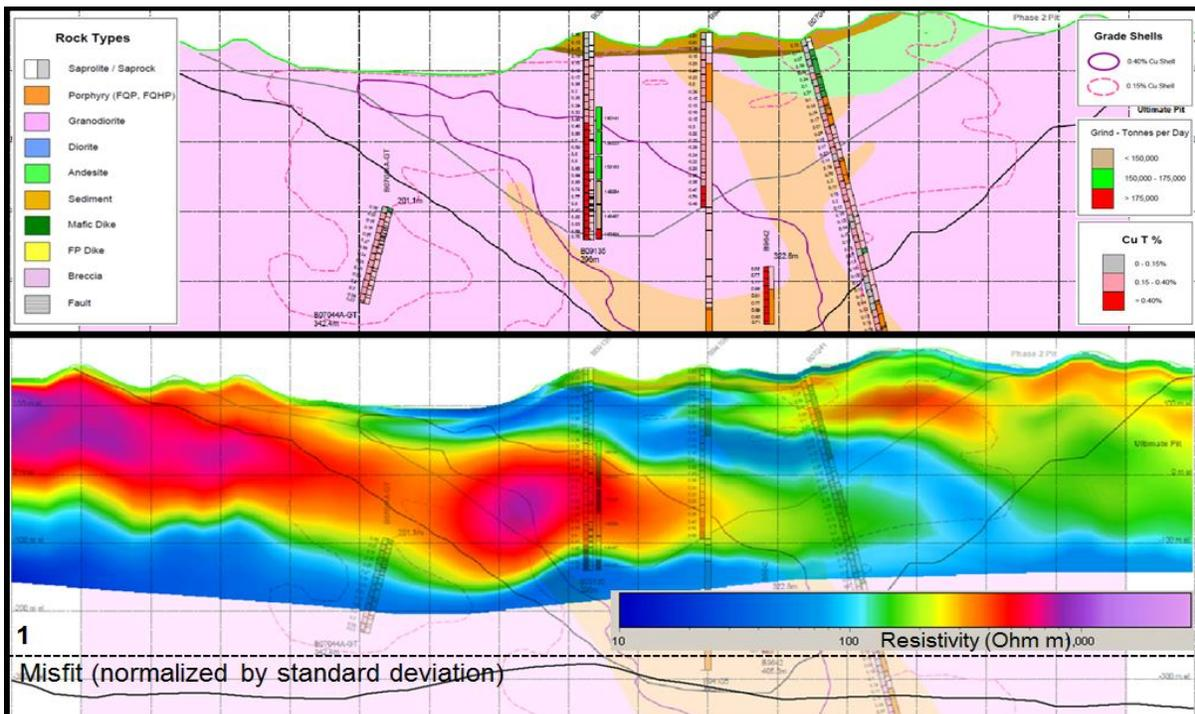
Figure 4 Inversion results over SkyTEM line 120801. Top: geological model constructed based on drilling information with contours of projected open pit mine; bottom: resistivity depth section derived from SCI inversion.
