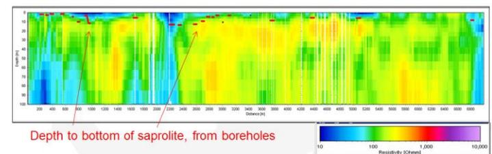
**Figure 2.** Example of the inversion results verified against the existing boreholes.
