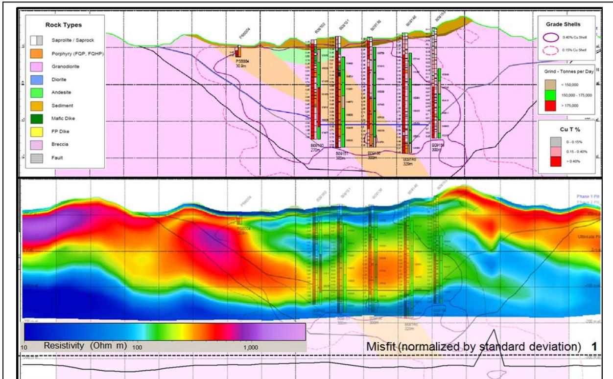
Figure 3. Inversion results over SkyTEM line 121801/121802. Top: geological model constructed based on drilling information with contours of projected open pit mine; bottom: resistivity depth section derived from SCI inversion.
