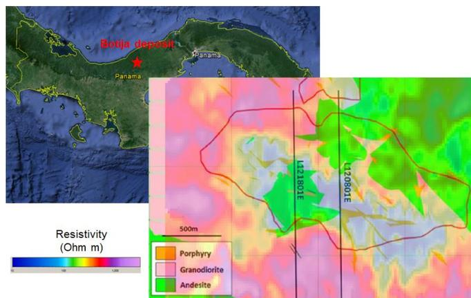
**Figure 1.** Location and simplified geology of Botija Cu porphyry deposit, Panama, showing SkyTEM flight lines 120801 and 121801 and overlain by recovered electrical resistivity, gridded at 30-40 m below surface.
